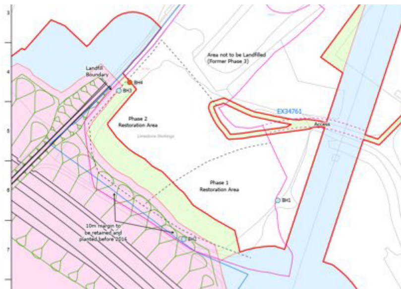
Plate G.7 Plan showing Project land requirements overlaid with Tarmac permit area and boreholes
